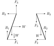
The surface is high friction, so  $F_1$  and  $F_2$  can be arbitrarily large. Slipping can only occur at the apex. Assuming limiting friction at that point,  $F_3 = \mu R_3$ . Taking moments around the base of the left-hand card,
