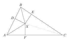
Triangles AFX and ADX are congruent, as are BDX and BEX. So, perpendiculars DX, EX, FX are all the same length. Triangles ECX and FCX are right-angled, with the hypotenuse CX in common and |EX| = |FX|. Hence, they are congruent, proving that CX bisects angle C. The angle bisectors are therefore concurrent.  $\Box$
