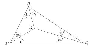
Angle RXQ is  $180^{\circ} - \frac{1}{2}\beta - \frac{1}{2}\gamma$ . Since the lines of action meet at X, this is the obtuse angle between the forces at R and Q meeting tip-to-tip. So, the acute angle between the forces at R and Q meeting tip-to-tail is
