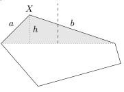
Move X onto the dashed perpendicular bisector, leaving the other vertices where they are. Since the total length a + b is fixed, this must increase the perpendicular height h of the shaded triangle, thus increasing its area. Hence, the new pentagon has a greater area than the original one. This is a contradiction. Therefore, for a fixed perimeter P, the pentagon of greatest area is regular.
