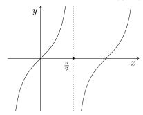
By symmetry and the shape of the curve, the shortest path between these two branches must pass through  $(\pi/2, 0)$ , thereby having the form  $y = m(x - \pi/2)$ .
